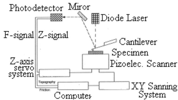
**Figure 2: Schematic of the typical AFM and its function**
