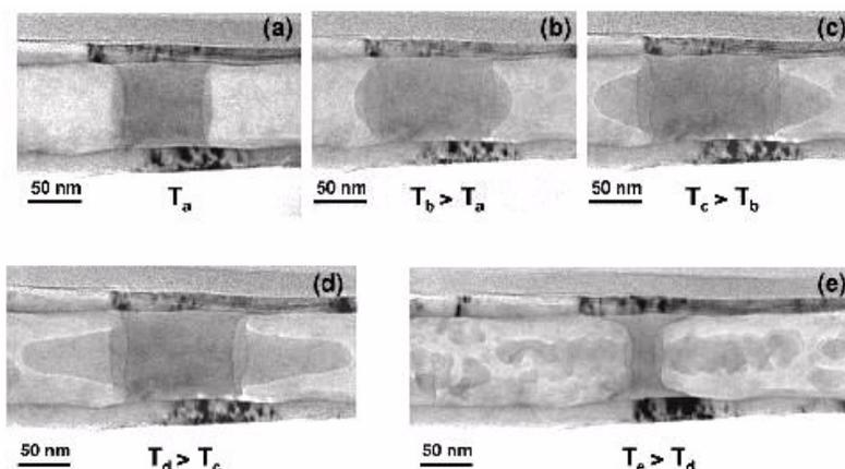
**Figure 5:** Complex temporal behavior of a water inclusion upon heating with the electron beam [23]: (a) initial state, (b), (c) expansion of the inclusion, possibly due to gas dissolution into the liquid under high pressure, (d) Formation of long tongue protrusions near the axis, and (e) disintegration of the inclusion and formation of a thin membrane. The observed events were irreversible after (b).
