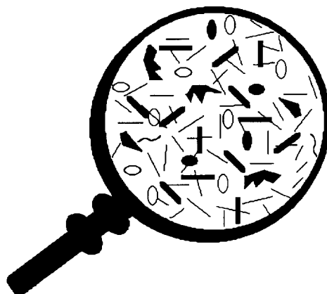
Fig. 1. Microscopic level composition of a petroleum crude containing heavy organics. In here straight and curved lines represent the paraffinic molecules, solid ellipses represent the aromatic molecules, open ellipses represent the resin molecules, and solid blocky forms represent the asphaltene molecules.
