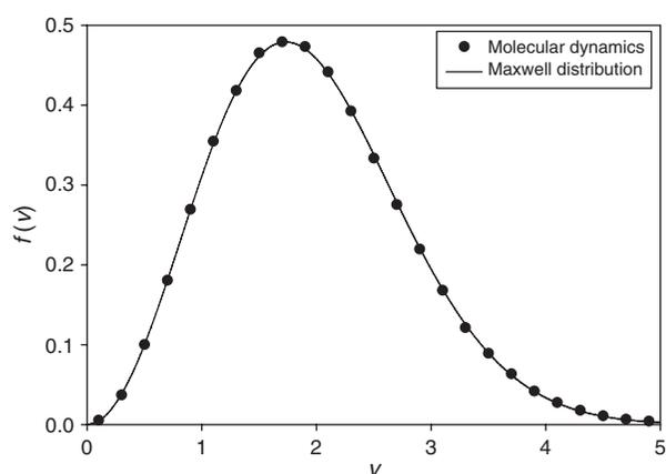
**Fig. 8.** Distribution of the atomic speeds for a system of 8 argon-like particles at  $T = 1.5$  and  $V/N = 1.5$ , both in reduced units. The solid line is the Maxwell distribution function at  $T = 1.5$ .
