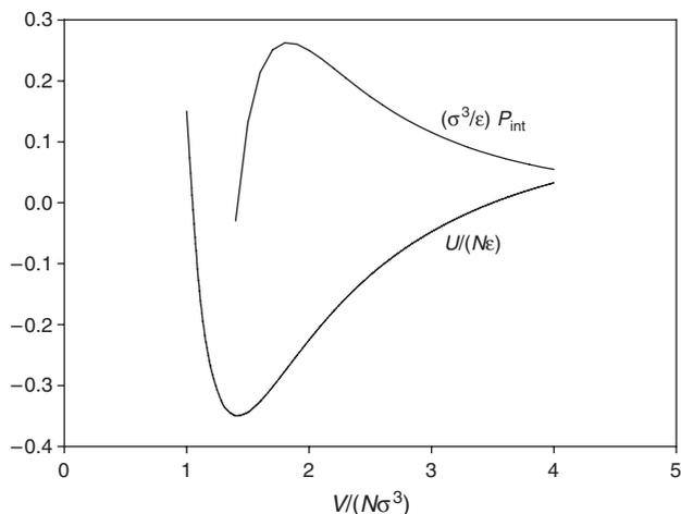
**Fig. 1.** Dimensionless plots of internal energy and internal pressure versus volume at constant temperature and particle number for a system obeying Lennard-Jones (6-12) potential energy function.
