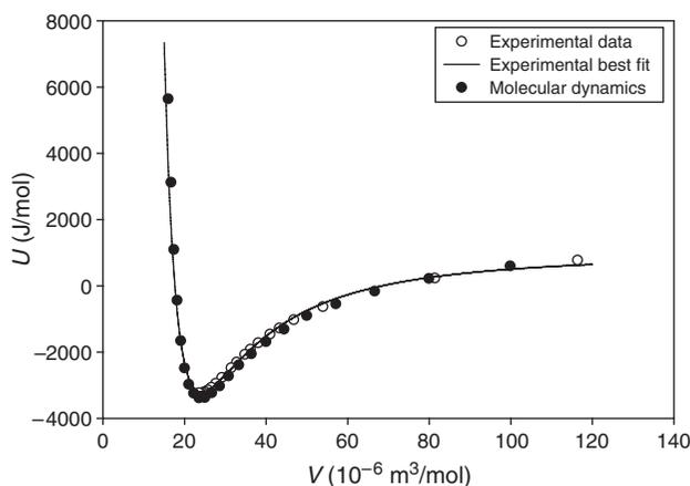
**Fig. 2.** Comparison between experimental data, their least-square fit, and molecular dynamics simulation of the internal energy of a macroscopic argon system at 180 K. The experimental data and the molecular dynamics simulations are from Goharshadi et al. Reprinted with permission from [16], E. K. Goharshadi et al., *Chem. Phys.* 331, 332 (2007). © 2007.
