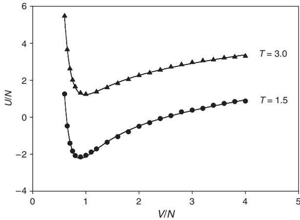
**Fig. 3.** Molecular dynamics data for the internal energy of 1000 argon-like particles as a function of volume at two different temperatures. The solid lines are the least-squares fits of the data to Eq. (33).
