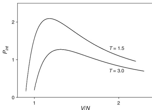
**Fig. 6.** Internal pressure for a system of 1000 argon-like particles as a function of volume at two different temperatures. The plots are calculated from the best fit of Eq. (33) to internal energy data in Figure 3.
