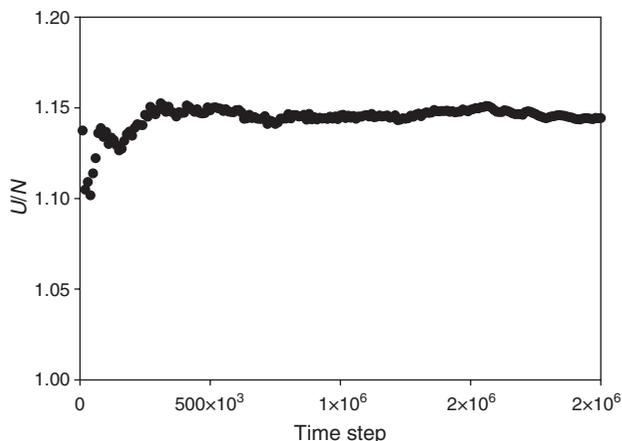
**Fig. 9.** Evolution of internal energy during the simulation of 8 argon-like particles at  $T = 1.5$  and  $V/N = 1.5$ , both in reduced units.
