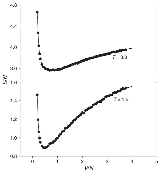
**Fig. 7.** Molecular dynamics data for the internal energy of 8 argon-like particles as a function of volume at two different temperatures. The solid lines are the least-squares fits of the data to Eq. (35).
