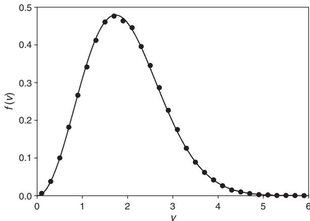
**Fig. 4.** Distribution of the atomic speeds for a system of 1000 argon-like particles at  $T = 1.5$  and  $V/N = 1.5$ , both in reduced units. The solid line is the Maxwell distribution function at  $T = 1.5$ .
