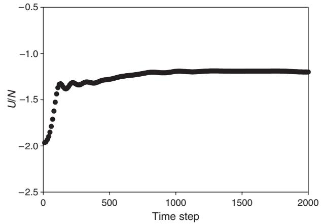
**Fig. 5.** Evolution of internal energy during the simulation of 1000 argon-like particles at  $T = 1.5$  and  $V/N = 1.5$ , both in reduced units.
