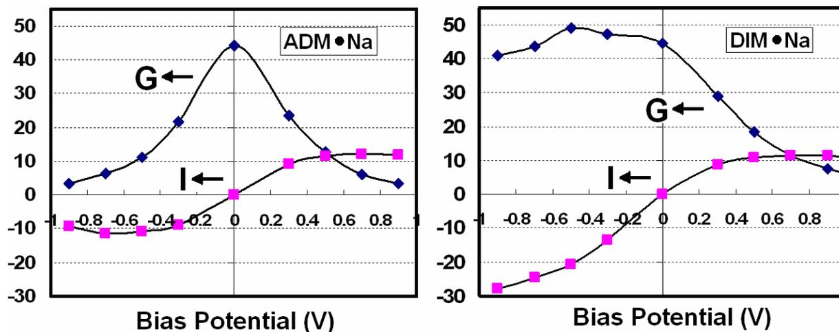
Fig. 4.  $G[\mu\text{S}]$  versus  $V[\text{V}]$  and  $I[\mu\text{A}]$  versus  $V[\text{V}]$  characteristics of ADM-Na and DIM-Na in linear electrodes corresponding to their horizontal orientations (Orientation 2 in Table 3).
