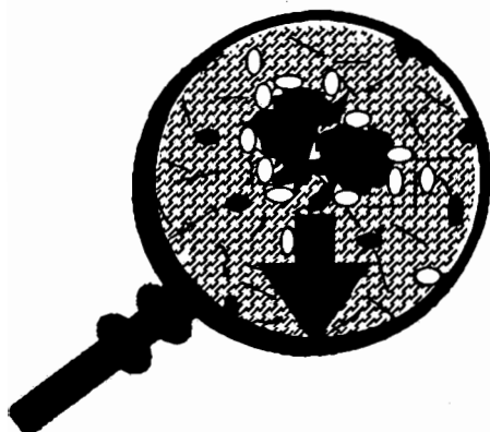
Figure 5: Flocculation and deposition (arrow) of very large heavy organic particles
