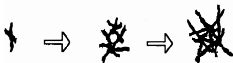
Figure 6: A possible growth pattern for asphaltene aggregates
