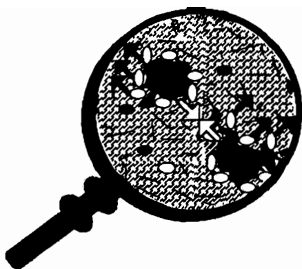
Figure 4: Migration of peptizing molecules (shown by black arrows) from the surface of heavy organic particles due to the change in their chemical-potential-balance between the bulk oil phase and the surface phase. This causes the potential for aggregation (white arrows) of heavy organic particles due to development of free active sites on their surfaces, and their eventual flocculation as shown below
