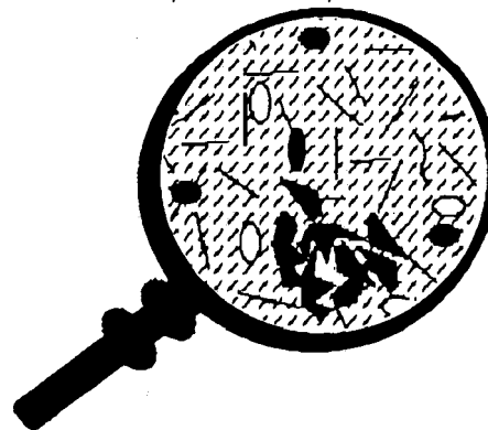
Figure 2: Flocculation and precipitation of the heavy components of a petroleum crude due to the introduction of a miscible solvent
