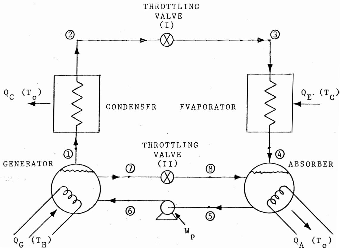
Fig. 3. Absorption Cooling Cycle.
