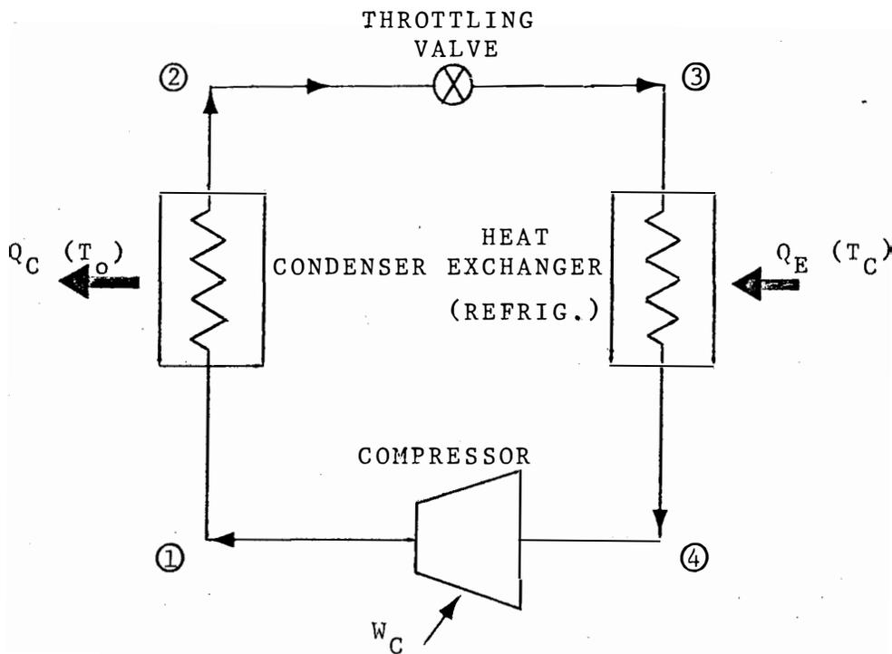
Fig. 2. Rankine Cooling Cycle
