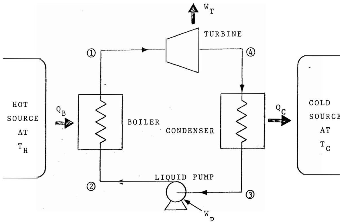
Fig. 1. Thermodynamic Power Cycle
