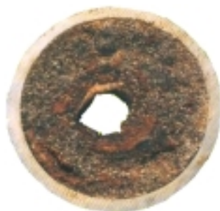
Figure 13 - Pipeline petroleum transport plugging due to wax and other heavy organics depositions (Courtesy of Phillips Petroleum Company)
