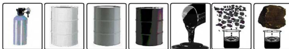
Figure 18 The normal conditions of the seven naturally occurring petroleum fluids, in the order of fluidity from left to right, natural gas, gas-condensate (NGL), light crude oil, intermediate crude oil, heavy oil, tar sand and oil shale (see online version for colours)
