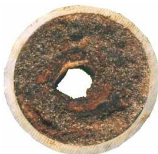
Figure 12 Pipeline petroleum transport plugging due to wax and other heavy organics depositions (see online version for colours)
